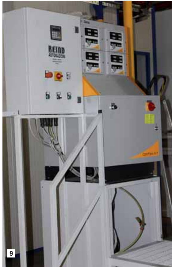
9 The control panel of the reciprocators and of the guns by Gema Europe.
