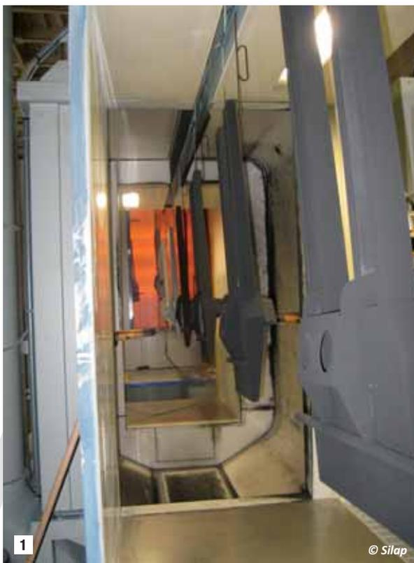
**1** *Some three-dimensional steel sheet parts hanging from the UV-curable powder coating plant. The UV system with reflectors developed by Euroimpianti ensures the perfect polymerisation of the film on the workpiece, even in the undercuts.*
