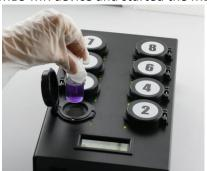
The MBS-MR device consists of 8 independent stations that allow the simultaneous execution of multiple tests. The analyzes are carried out using an optical thermostat reader which automatically detects the color change of the test vials and calculates the microbial concentration of the sample. Through the MBS-MR software, the test results are available and can be consulted within a database even during the execution of the test.
