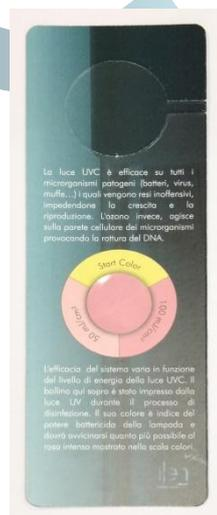
In this way it is possible to declare to have subjected the surfaces to UVC treatment with a dose of UVC like that indicated by the color of the DOTS
